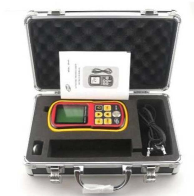
**Gambar 3.7 Ultrasonic Thickness Gauge**
